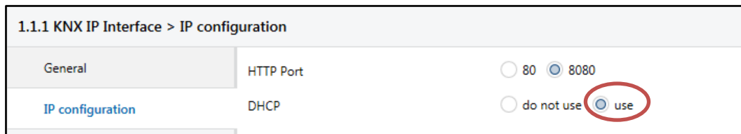
Figure 6: IP Configuration Tab Parameters, DHCP on
