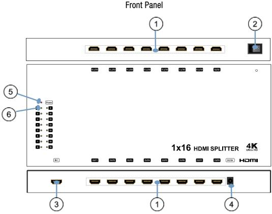
1) HDMI outputs. 2) Power on/off: press the up/down to open/close the device.
